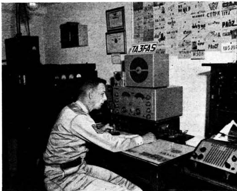
TA3FAS—ANKARA, TURKEY Society member, Jim Fry, W5HBQ—depicted here—is the present operator at TA3FAS. The main receiver is a National NC183, and the two transmitters are BC610s, one for 14 and 28 Mc/s., and the other for 1.7, 3.5 and 7 Mc/s. Four element beams are used for 14 and 28 Mc/s., and a 275ft. long wire for the other bands. TA3FAS will be active shortly on 1,900, 3,510 and 3,520 kc/s.
